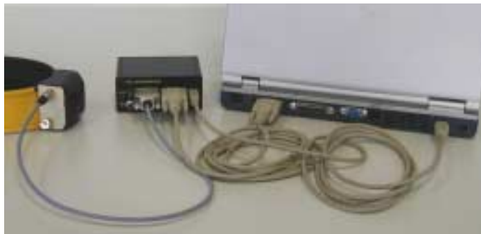
Figure 7: RS232 and USB connection between Collar and PC/Laptop via LM1
