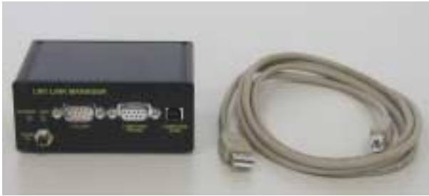
Figure 4: Connection between PC/Laptop and LM1 with an USB cable
