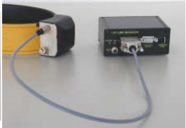
Figure 5: Connection between Collar and LM1 with the special link cable
