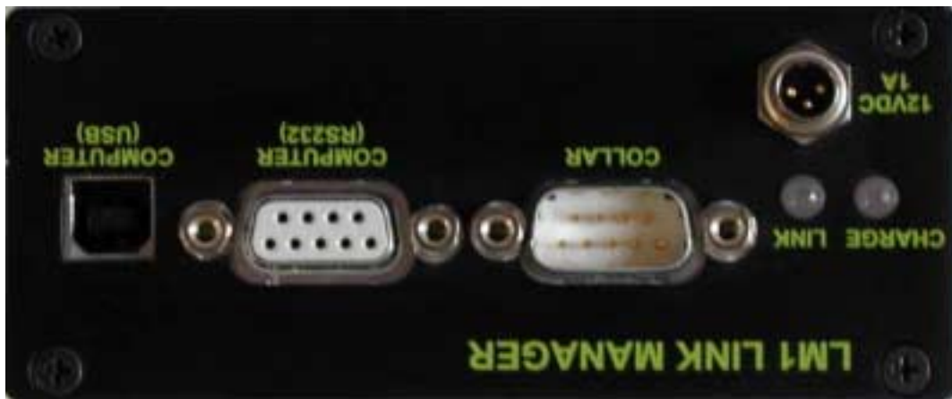
Figure 9: LM1 turned upside down to reset the battery protection circuit
