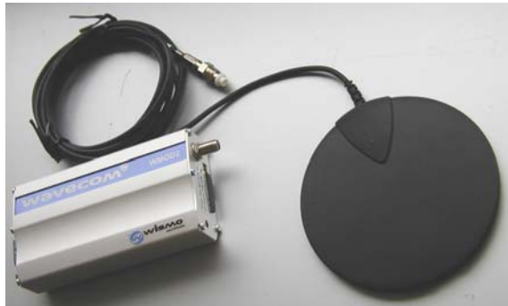
Fig. 3: The GSM groundstation is best positioned near the computer. The position data arrive from the collar via SMS.
